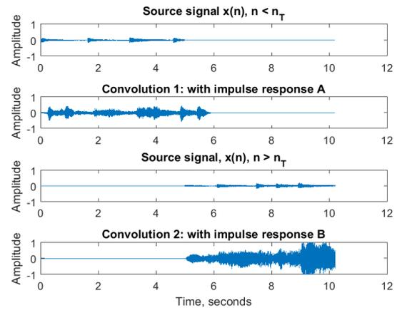
Figure 6: Convolution demonstration: Two overlapping time-invariant convolutions. Upper pair: Source signal segment for  $n < n_T$  followed by the convolution with impulse response  $h_A(n)$ . Lower pair: Source signal segment for  $n \geq n_T$  followed by the convolution with impulse response  $h_B(n)$ .
