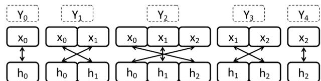
Figure 2: Example of partitioned convolution with 3 partitions [8]
