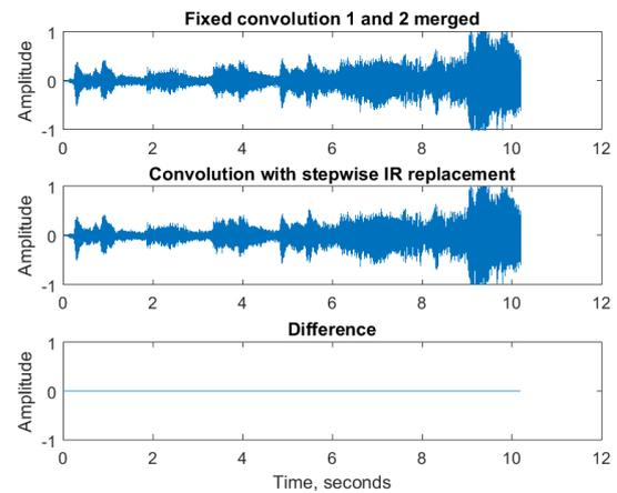
Figure 7: Convolution demonstration: Comparing time-variant method with two overlapping time-invariant convolutions. Top: The merged result of the two time-invariant convolutions in figure 6. Middle: The output when using stepwise IR replacement. Bottom: Difference between the two.
