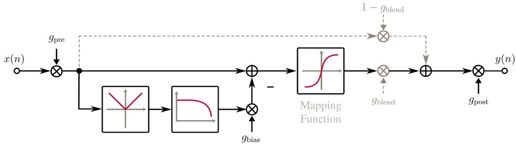
Figure 2: Signal flow graph of a nonlinear block. Blend stage is omitted in the second nonlinear block.
