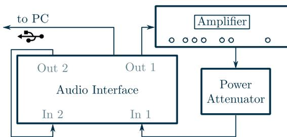
Figure 4: Measurement Setup.
