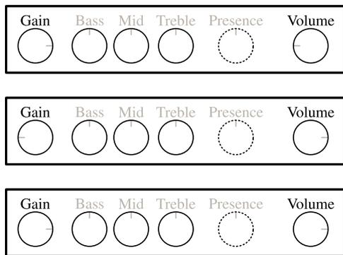
Figure 7: Settings for pre-amp distortion (top), power-amp distortion (middle) and heavy distortion (bottom).
