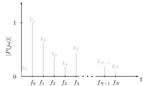
Figure 3: Overtone of a sinusoidal signal after the polynomial mapping function.
