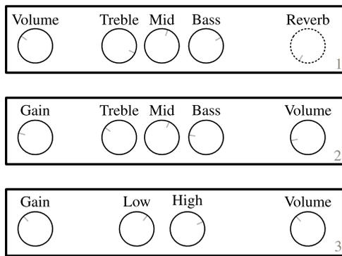
Figure 6: Settings for amplifiers in clean setting. 1.) Ampeg VT-22 (top) 2.) Fender Bassman 100 (middle) 3.) Fender Bassman 300 (bottom)
